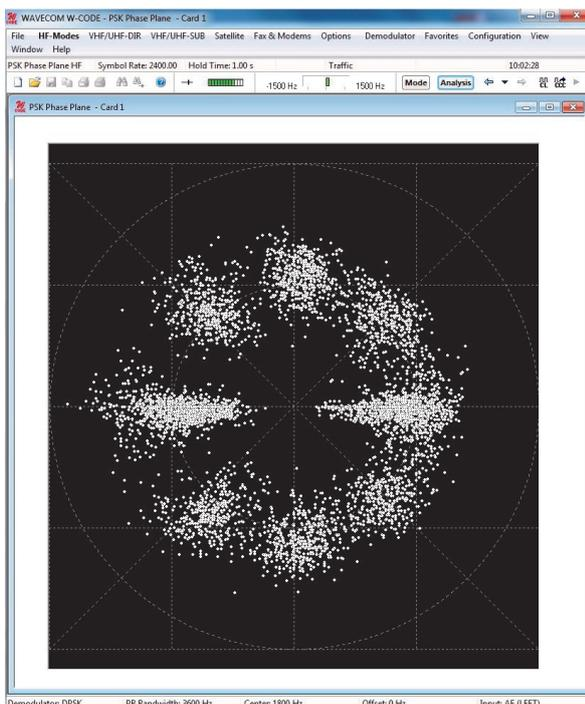
The screenshot to the left shows an AF recording of a STANAG-4285 signal using W-CODE and a PC sound card. The loss of quality due to the action of the sound card is clearly to be seen and will significantly degrade any subsequent decoding.
