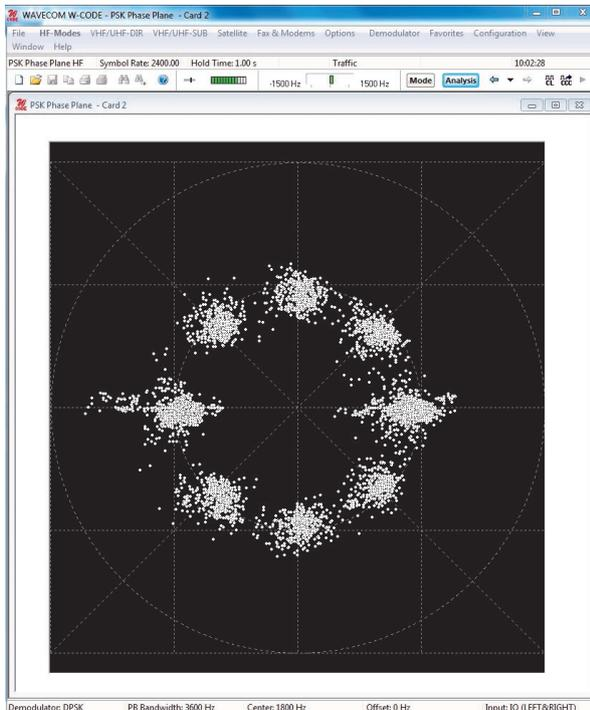
The screenshot to the left shows the high quality of an I/Q recording of a STANAG-4285 signal using W-CODE and a G39DDC SDR. The quality is as good as the conditions in the HF band allow. The signal arrives at the demodulator and the decoder with optimum quality.
