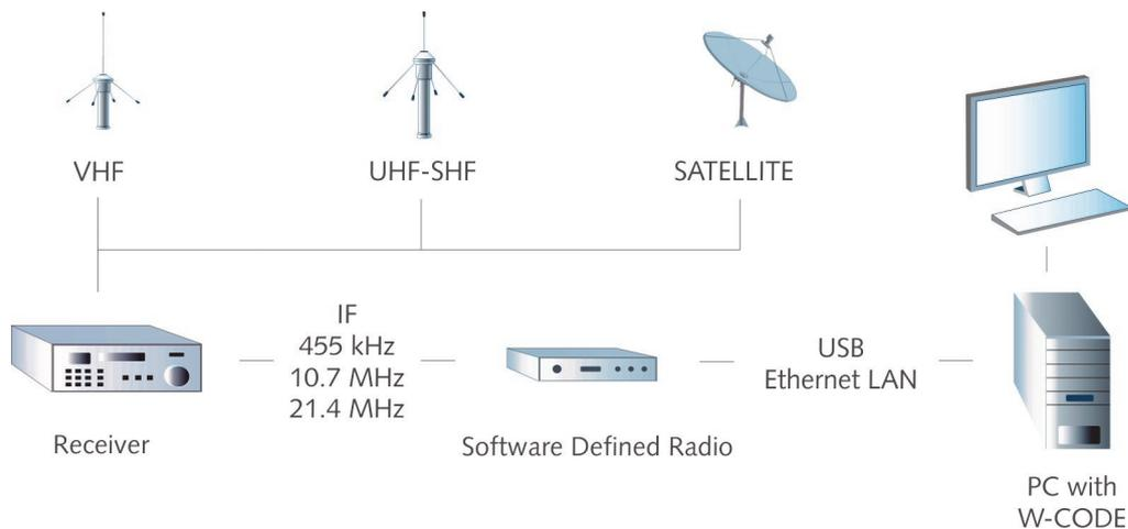
This setting uses an SDR (Software Defined Radio) receiver and W-CODE. In this example we are using the RF Space SDR-IQ receiver. The SDR-IQ has an input frequency coverage of 10 kHz to 30 MHz. Since the VHF/UHF-DIR transmissions are taking place above 30 MHz, an analog receiver must be used to downshift the signal into the range below 30 MHz. The receivers described in Setting 1 with an IF output frequency of 10.7 MHz are therefore suitable.
