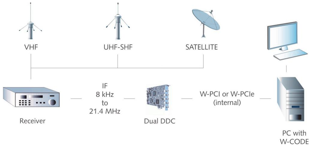
This setup includes an analog VHF/UHF receiver and the W-PCIe or W-PCI. We use receiving and decoding TETRA as an example. Allocated frequencies for TETRA systems are in the VHF band, therefore a VHF analog receiver is needed to downshift the actual transmission frequency to a fixed output IF frequency which is supported by the W-PCIe (12 kHz-25 MHz). Commonly available VHF receivers have an IF output frequency of 10.7 MHz (wideband) or 455 kHz (narrowband).
