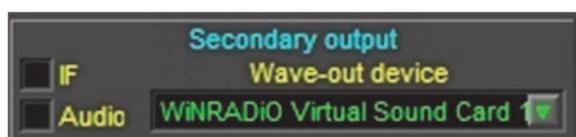
The secondary output is particularly useful in conjunction with the optional WiNRADiO Virtual Sound Card software, which makes it possible to pass the digitized signals from the receiver directly to a third-party application without any intervening re-digitization process, and therefore without intro-
