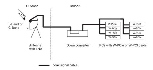
The monitoring system consists of three main components
