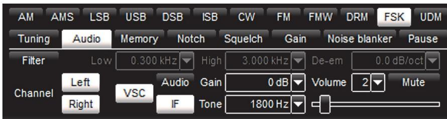
Select in W-CODE "Configuration -> W-CODE Device..", and "Input: IQ (Left & Right)" for decoding and analytic functions. Once these steps have
