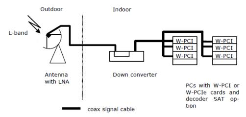
The monitoring system consists of three main components:
