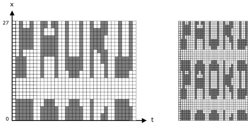
As shown on the left side illustration above, the message text will be cut and shifted. There is no synchronization marker in a FELD-HELL or FM-HELL radio signal, thus it is impossible to avoid this problem while decoding the signal. The easiest solution is to display the image twice, one below the other, as shown on the right side illustration.
