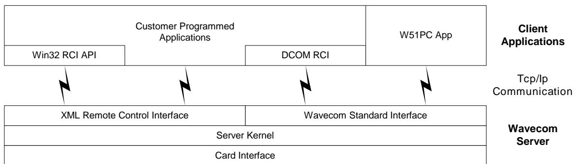
WAVECOM provides two remote control interfaces based on a client-server architecture:
