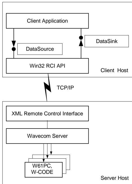
Procedural (C) and object oriented (C++, C#) interfaces are defined for the Win32 Remote Control Interface API. The sink (callback) must be programmed by the client application programmer - a function type definition for the C API and a virtual parent class for the C++ API is available for the sink. The sink implementation must be passed to the API before starting communicating with a server.
